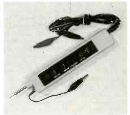
FIG. 2—GLOBAL SPECIALTIES' LP-2 logic probe, like most others, derives its power from the circuit under test through clip leads (top).
