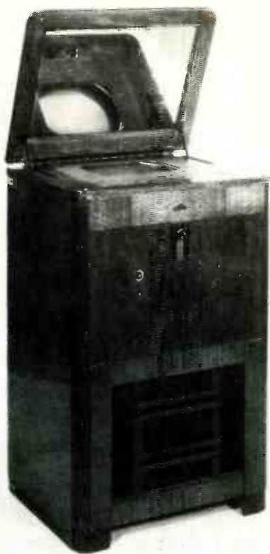
FIG. 2—ONE OF THE LAST in existence, this receiver was one of the ones used in RCA's test of the first all-electronic television system. The vertically-mounted picture tube was viewed through a mirror in the cabinet top.
